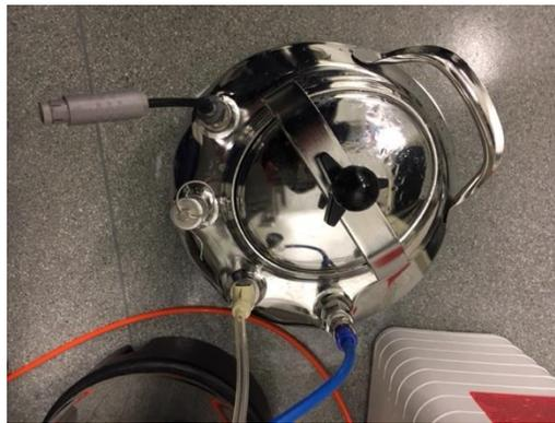
7. Fill the Sheath Tank with sterile PBS 1X under the hood and empty the Waste Tank and fill it with a little bleach
